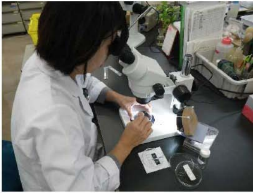
Figure 13: Separating Microplastics by picking and using the stereomicroscope (CMSM, 2018) Density
