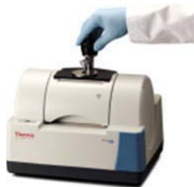
Figure 16: Nicolet iS5 FTIR Spectrometer with the ID7 ATR accessory in the sample compartment.
